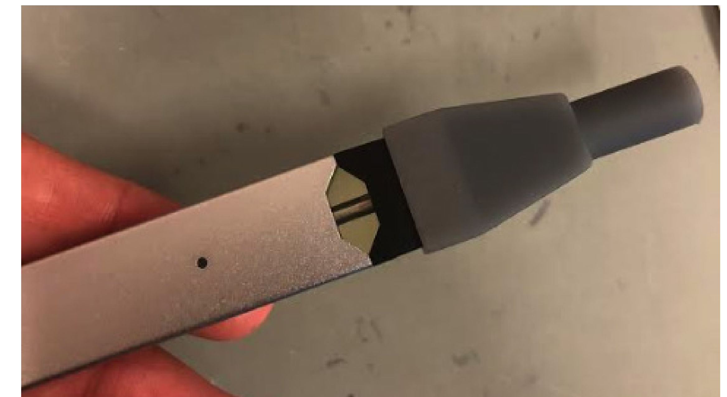
Figure 5: Final 3D-printed conduit device for use with VitroCell VC10 Smoking Robot. Heat stable resin with a 0.09mm midline channel for JUUL vapor.
